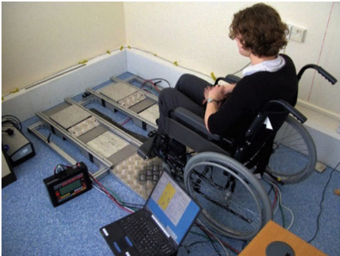
Fig. 13.1 A load-cell based wheelchair assessment system
