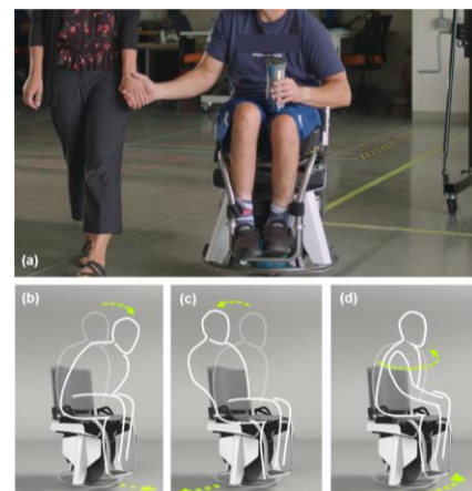
Figure 1. Novel wheelchair (PURE) uses torso motions for (a) hands-free control to move omnidirectionally: (b) forward-backward, (c) sideways, and (d) spin in place.
