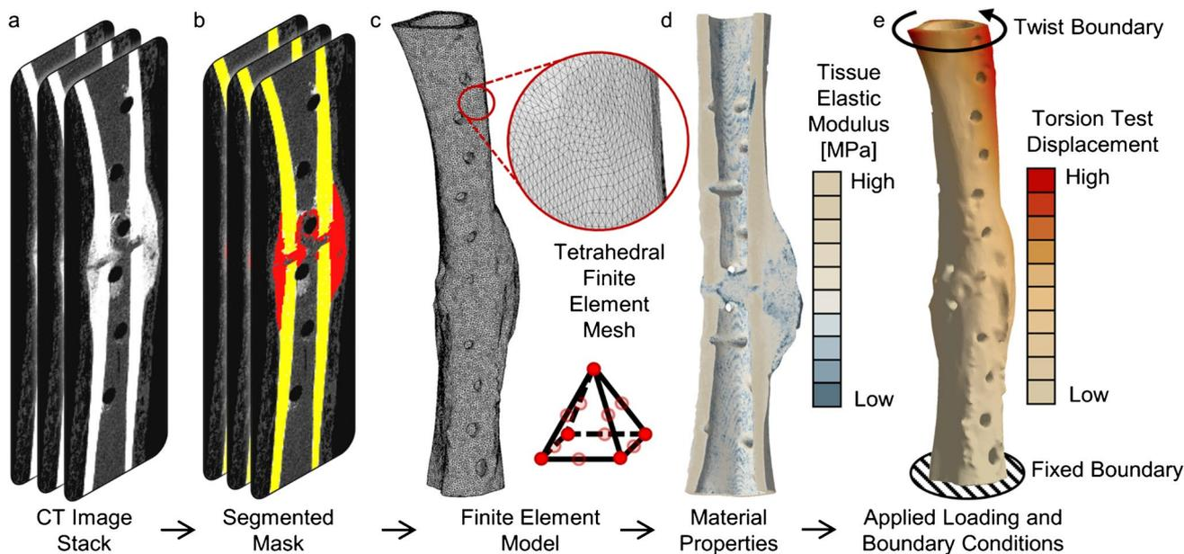
**Fig. 2** General procedure for image-based finite element (FE) modeling illustrated for a healing ovine osteotomy [16]. (a, b) CT image stacks are segmented to identify the bone geometry. The volume is then meshed (c), shown here using tetrahedral finite elements. (d) Local material properties are interpolated and scaled from the radi-
