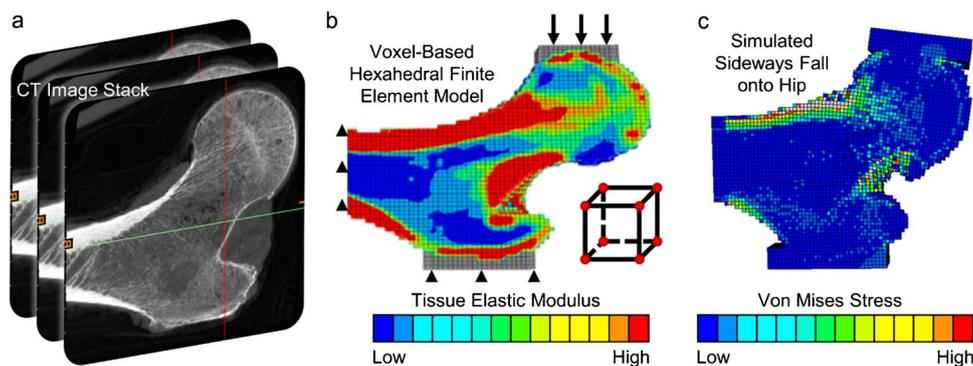
**Fig. 4** Example of a proximal femur that is directly converted from a CT image to an FE model with hexahedral elements. (a) The region of interest is segmented from the CT image stack and resampled to create isotropic voxels. (b) Voxels are directly converted into linear hexahedral elements and assigned density-based material properties. Because the mesh itself is rather simple, more complex material
