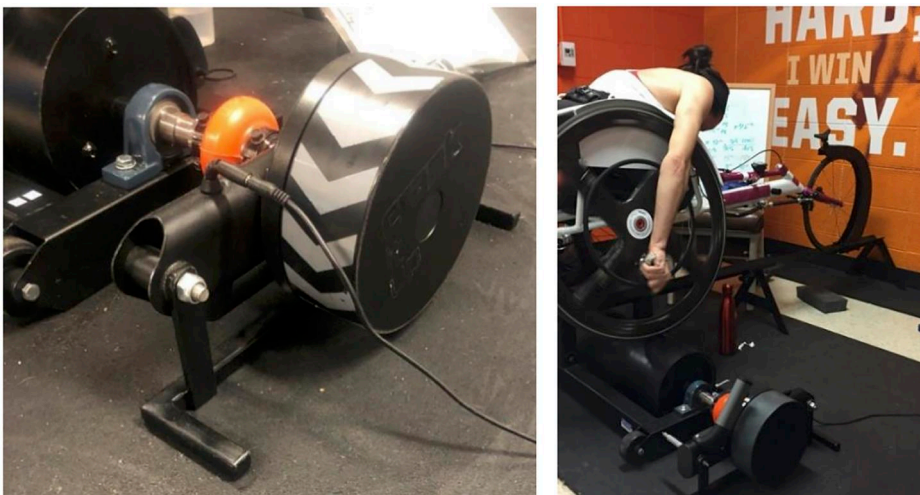
Figure 4. An electromagnetic resistance flywheel adapted and coupled to a free-spinning indoor roller (left) and an athlete using the smart roller while practicing (right).
