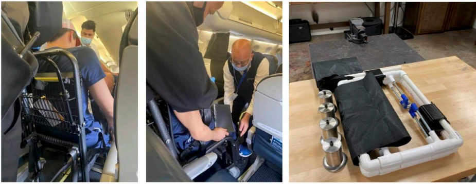
Figure 6. An individual transfers from airplane seat to aisle chair to move down the aisle and get off the airplane (left). The individual is not able to move independently and must rely on attendants (middle). A new design will allow individuals to easily carry and deploy a personal aisle chair for use, providing them independence while traveling on an airplane (right).
